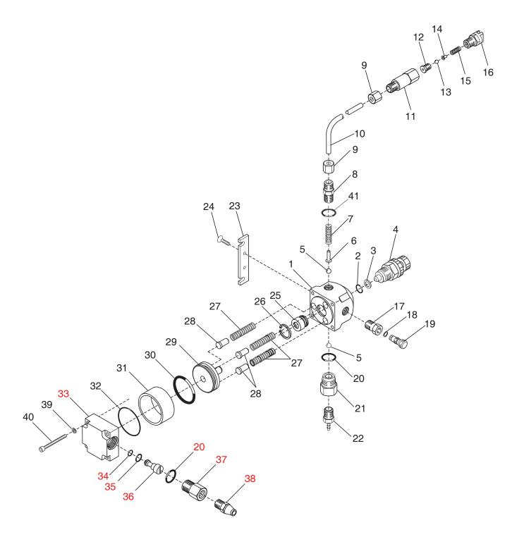
NOTE: ITEMS MARKED (\*\*) ARE AVAILABLE IN A REPAIR KIT UNDER THE PART NO. 210-ACY-01 NOTE: ITEMS MARKED IN RED ARE AVAILABLE AS AN ASSEMBLY UNDER PART NO. SP0210VAL01
