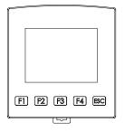
A solid-state programmable Actuator. It is activated by a proximity sensor that sends a signal to a solenoid to trip the MicroSpray
