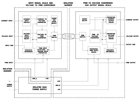
**Applications:** The signal converter provides precise signal conversion and isolation between sensors, PLC's and other controls. Applications include industrial automation, test equipment and off-highway machine automation. For harsh environments, the module should be mounted in a protective control panel.
