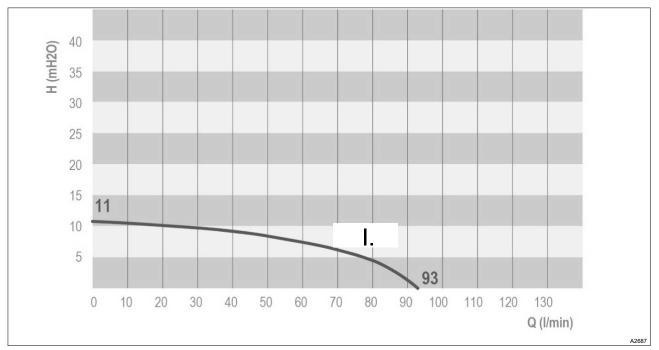
*Fig. 12: Performance diagram. Measured values* ± 5 %*, test medium: water 20 °C, 1" pressure pipe, oval wheel meter.*
