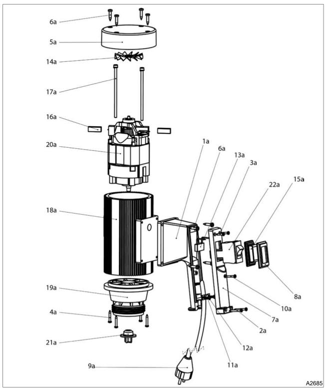
Fig. 9: Spare parts drawing for the motor.
