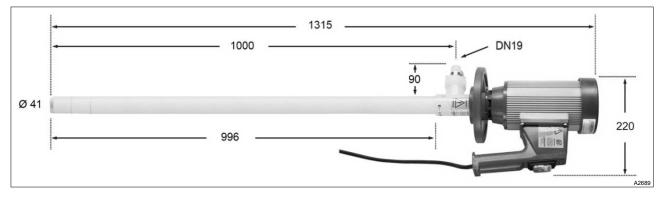
Fig. 14: PVDF version: Dimensional drawing with main dimensions, all measurements in mm.
