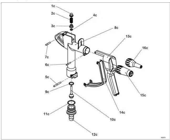
Fig. 11: Spare parts drawing for the pump nozzle.
