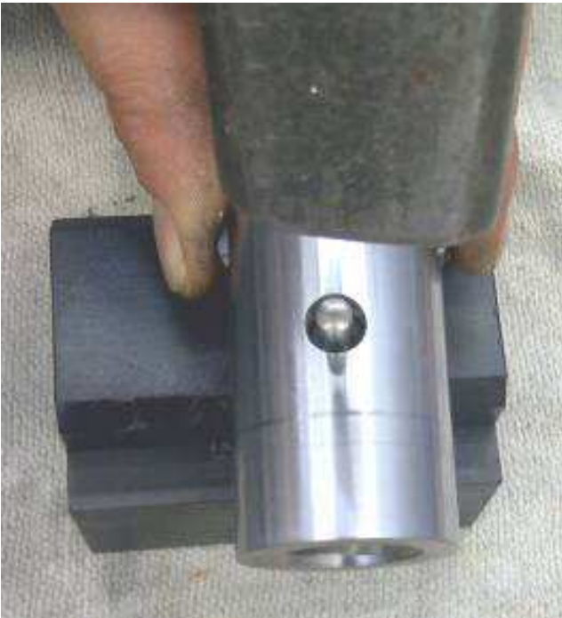
While the pin is mounted with a hammer, always make sure that the two fingers do move well
