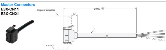
\* E3X-CN11: 4 dia. cable / 3 conductors / Standard length: 2 m (Conductor cross section: 0.2 mm² (AWG24), Insulator diameter: 1.1 mm) E3X-CN21: 4 dia. cable / 4 conductors / Standard length: 2 m (Conductor cross section: 0.2 mm² (AWG24), Insulator diameter: 1.1 mm)
