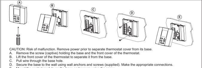
E. Mount the control module on the base and secure using the screw.
