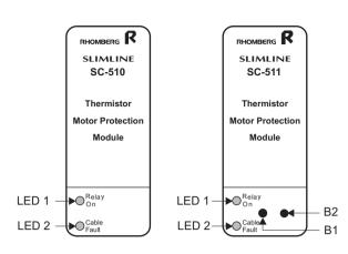
LED1: The LED marked "Relay ON" illuminates when the relay is energised.
