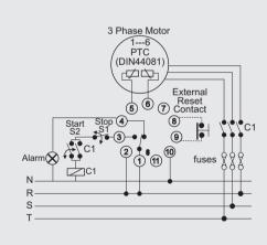
**APPLICATION 2** Three phase motor with PTC (DIN 44081)(SC-511)
