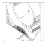
Blade-jaw distance of 2/13.5 mm Limits vibration and tube distortion
