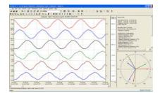
Real Time "Scope Mode" Waveforms and Phasor verification via PAS<sup>™</sup>
