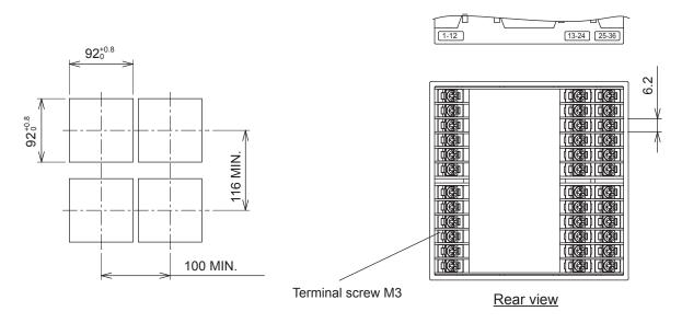
Terminal block is not attached to unused terminals (terminal 13 to 24) according to the model.
