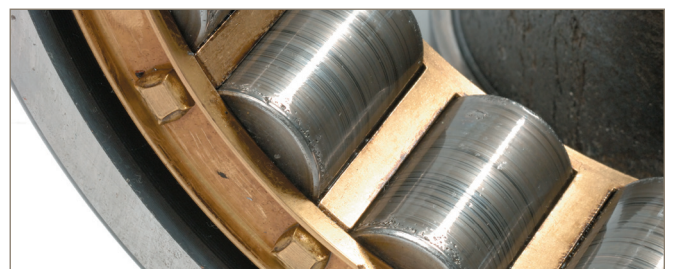
Examples of damaged gear wheel and roller bearing
