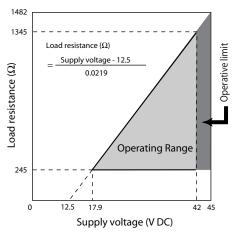
Figure 5 Supply voltage vs. load resistance characteristics
