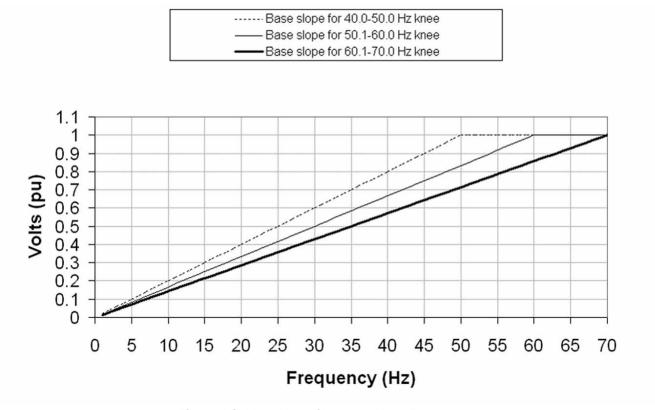
Figure 4-2. Volts/Hertz Slopes vs. Knee Frequency
