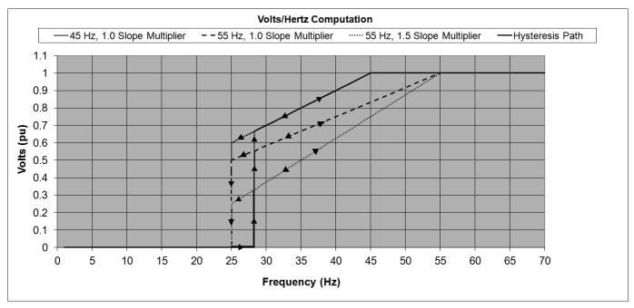
Figure 4-3. Examples of Under Frequency and Slope
