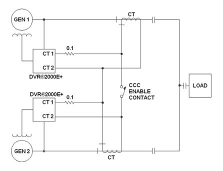
Figure 5-12. Cross-Current (Reactive Differential) Connections for Two Generators
