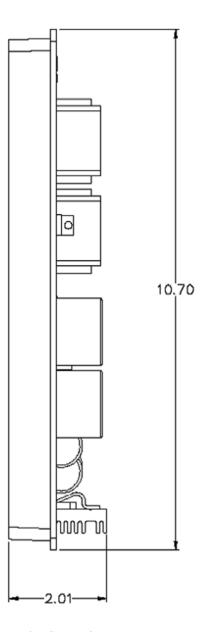
Figure 5-1. DVR® Front dimensions without cover. Valid for E+ & EC+ versions.
