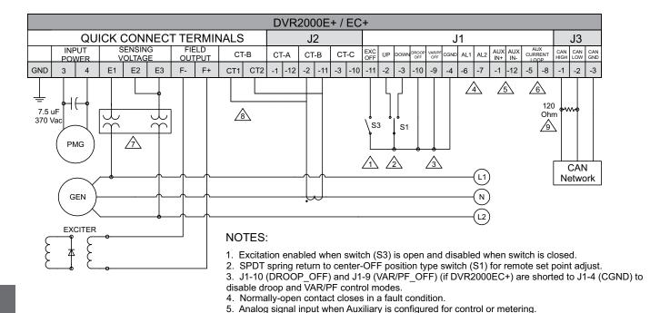
6. Should be shorted when Auxiliary is configured for 4-20 mA control or metering.
