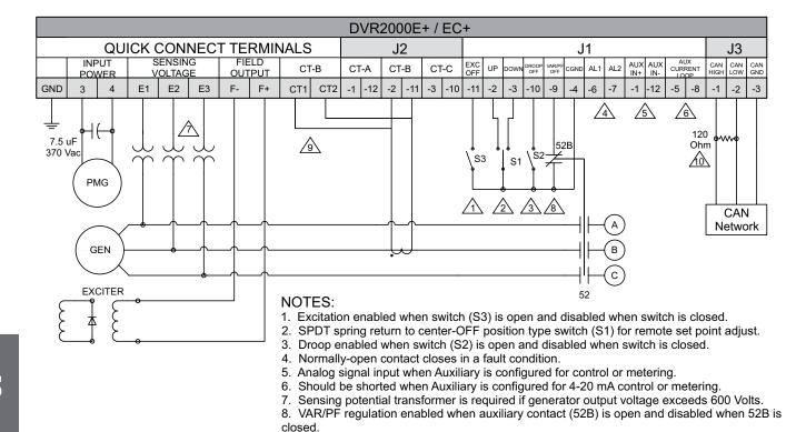
Figure 5-9. Typical Connections with ABC Rotation, Three-Phase Voltage Sensing and Single-Phase Current Sensing
