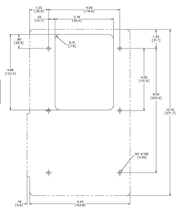
Figure 5-3. Cutout and Drilling Dimensions
