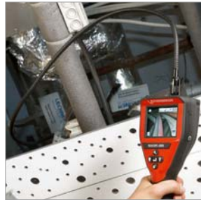
Camera head with high-performance LEDs
