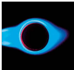
High flame temperature through cyclone swirl
