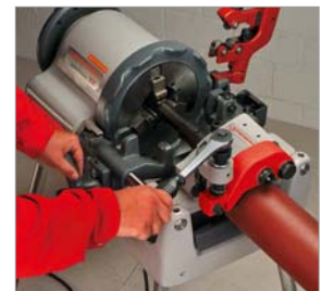
Cost-effective production of grooves
