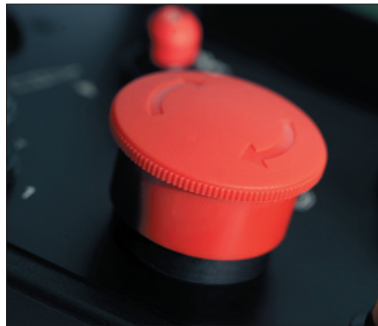
Activation of the stop button puts the system in a safe stop mode within 0.5 seconds.
