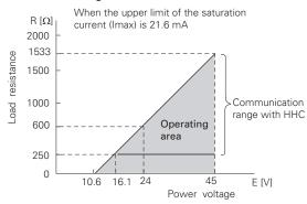
Note) The load resistance varies with the upper limit of the saturation current [I max]
