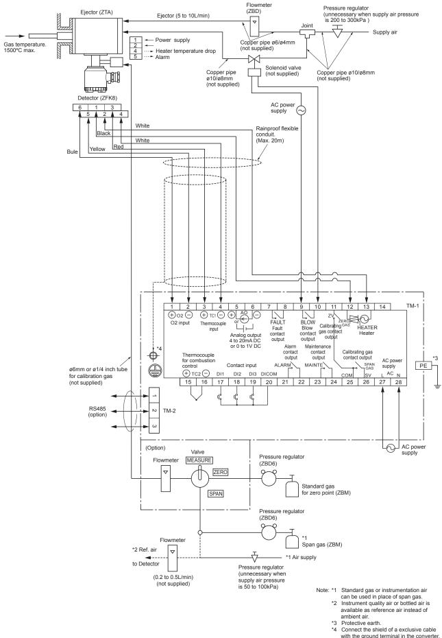
with the ground terminal in the converter. \*5 HART communication (option) uses a 4-20mA analog output terminal. Ejector system
