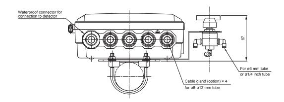
Converter (ZKMB) <IP67 enclosure> with selector valve and flowmeter
