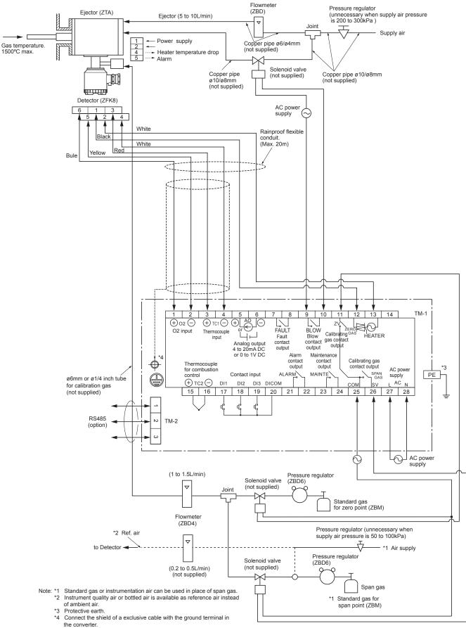
\*5 HART communication (option) uses a 4-20mA analog output terminal.
