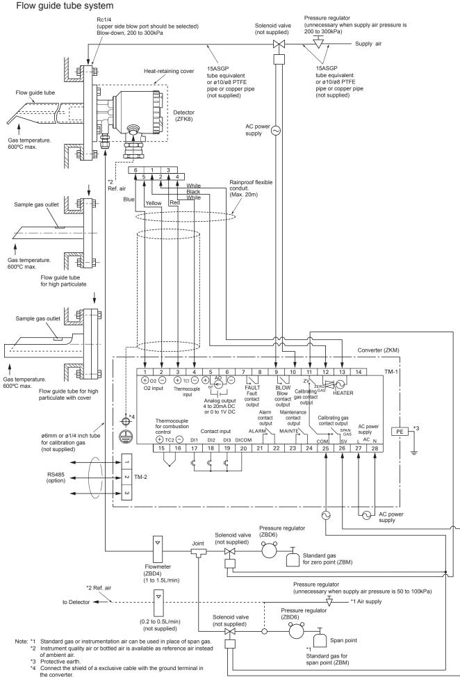
\*5 HART communication (option) uses a 4-20mA analog output terminal.
