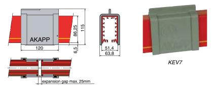
The rubber sealing at the inner side of the synthetic expansion joint clamp, together with the continuous AS7 sealing strips, also allows **installations outdoors**.
