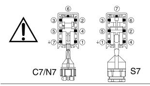
Trolley type S7 has different cable numbering.
