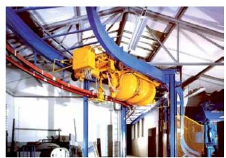
Feed and control of a concrete skipper
