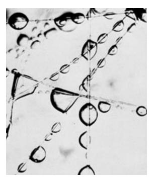
Photomicrograph of coalescing process inside fiberglass media.
